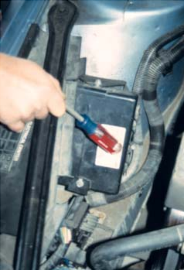
Figure 26–18 Tap testing a vehicle computer. General Motors recommends that only the four fingers of an open hand be used to tap test any component to avoid causing damage.
