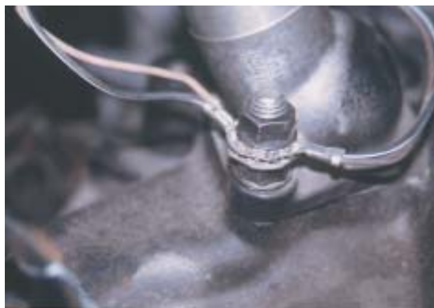
Figure 26–17 Always check that the computer grounds are clean and tight.
