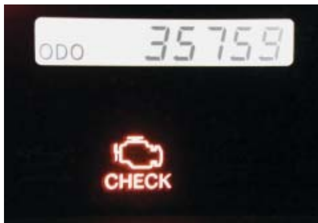
Figure 26–1 A typical malfunction indicator lamp (MIL), often labelled “Check Engine” or “Service Engine Soon.”
